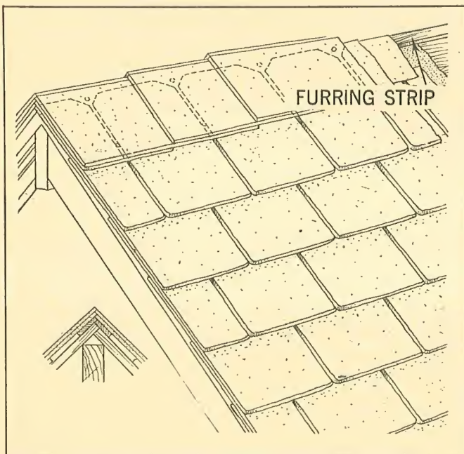
Figure 22—Boston Ridge construction
